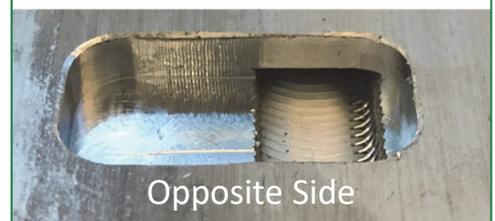
As a solid state fabrication technology, SBT FSP offers new benefits in the production of components having internal channels to meet internal fluid and gas flow requirements. Due to relatively low out-of-plane force applications, it is ideal for robotic applications, thereby opening up the possibility for producing low cost 5-axis internal pathways for wiring, fluids, gases, powders, etc.
