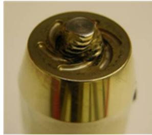
**Figure 5: Weld tool with the Wiper™ shoulder [10, 11].**
